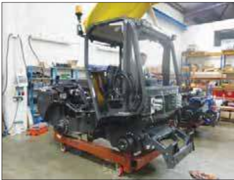
Cab joins the chassis after the hydraulics are in place
