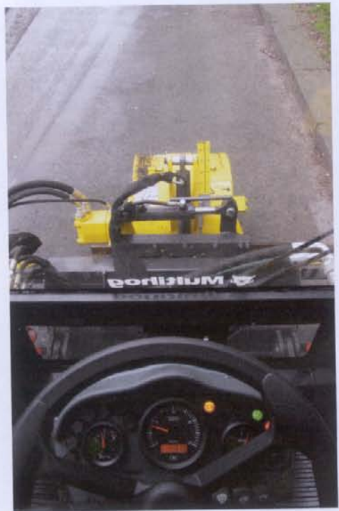
A major benefit with the Multihog is that the operator sits in an elevated position with a good view of the planer and the road surface.
